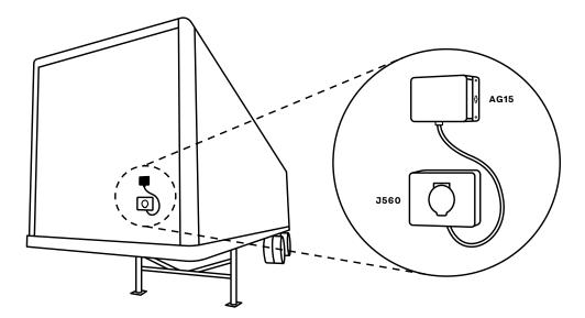
Dry van installation with power harness routed through J560's built-in cable grommet
