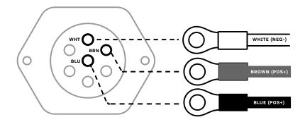
Note: Configuration of 7-ways can vary. Confirm color of connection before attaching lead. For install on trailers that require bullet connectors, please remove ring terminals and crimp the bullet connectors (included) to the wire ends.
